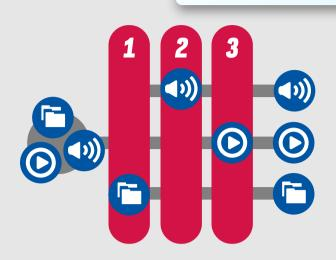
GPON separates data, voice and video onto three different network layers
